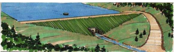
**AUXILIARY SPILLWAY (EMERGENCY SPILL- WAY)** - A secondary spillway designed to operate only during exceptionally large floods.
