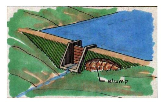
**SPILLWAY** - A structure over or through which flood flows are discharged. If the flow is controlled by gates, it is considered a controlled spillway; if the elevation of the spillway crest is the only control, it is considered an uncontrolled spillway.
