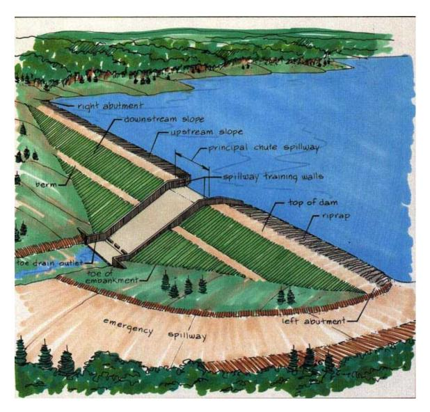
**SERVICE SPILLWAY** - A principal spillway used to regulate reservoir releases additional to or in lieu of the outlet.
