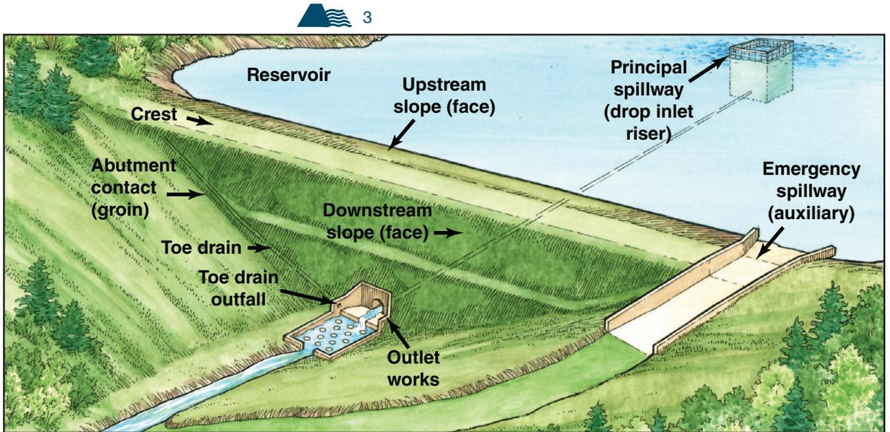
Figure 1—Typical dam diagram showing common terms.
