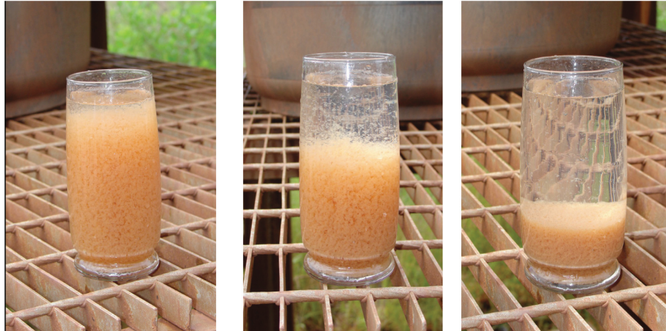
Figure 6.86a Flocculation of sediment with PAM.
