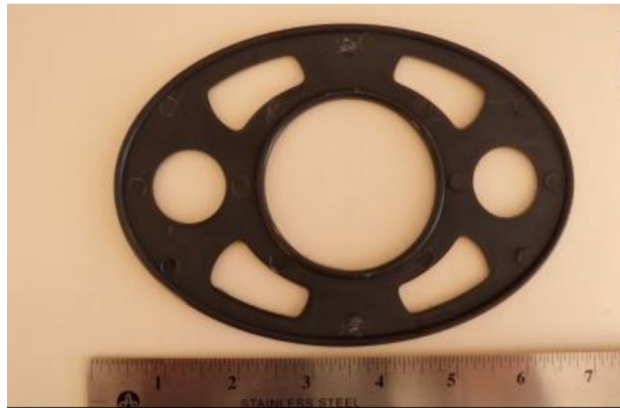
Figure 4.2.3. Polyhydroxyalkanoate biodegradable panel with cull ring and attachment points.
