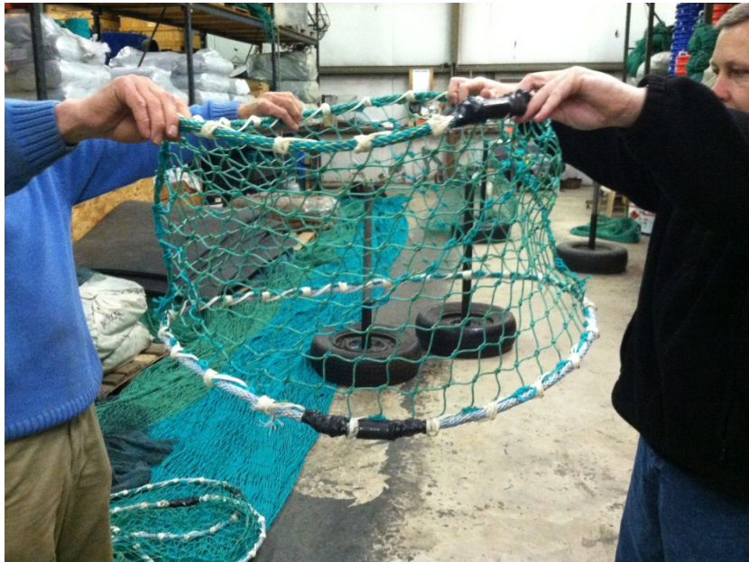
Figure 12.28 T90 extension constructed by Mikey Daniels.
