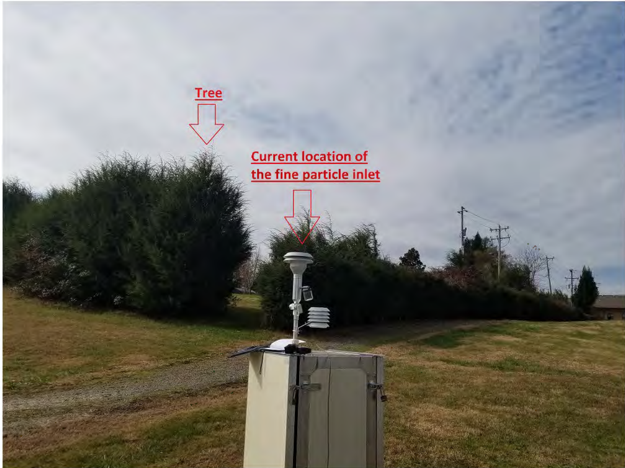
Figure 97. Current fine particle monitor location with trees in the background
