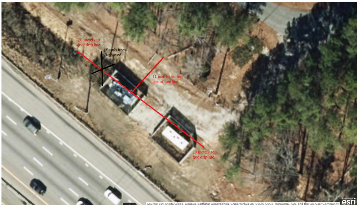
Figure 110. Site diagram showing locations of trees relative to the fine particle monitoring location.
