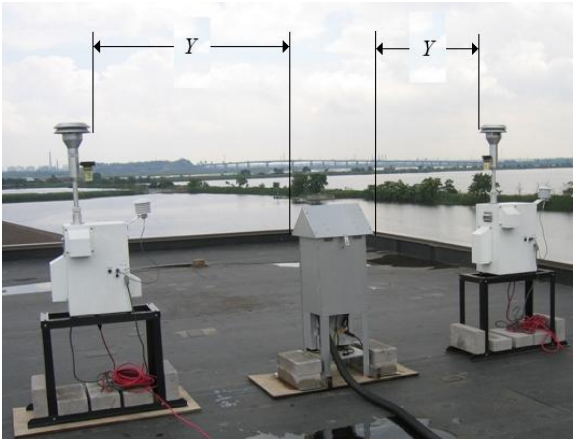
Figure 15. Measuring the Minimum Safe Spacing between Inlets
