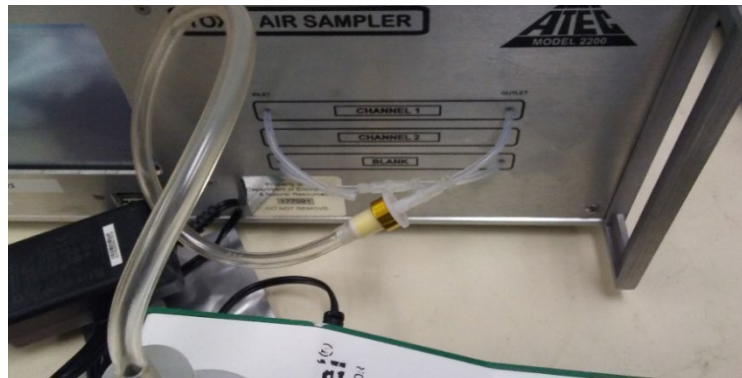
Figure 10: ATEC 2200 DNP Cartridge Flow Check Setup
