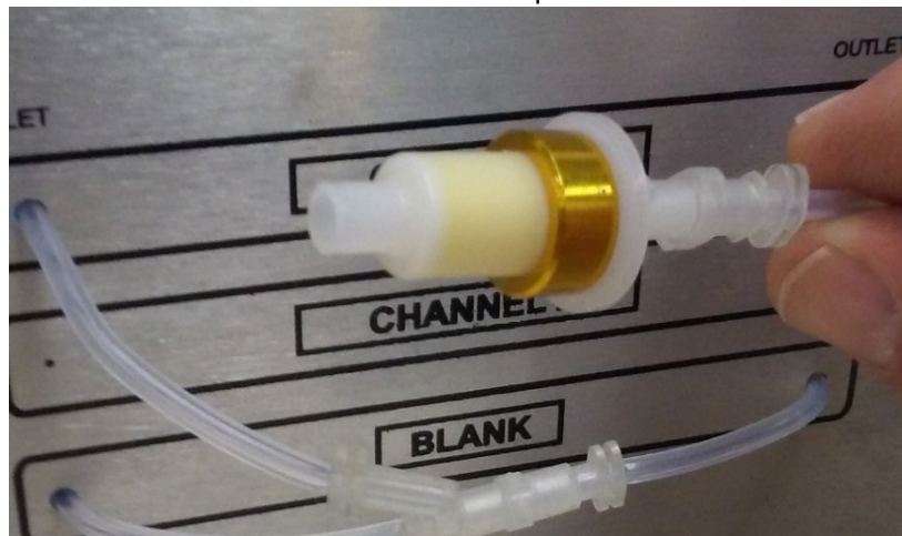
Figure 6: ATEC 2200 DNPH Cartridge Flow Check Connection Setup
