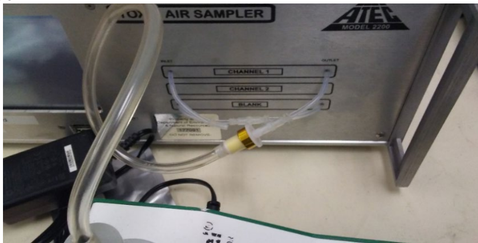
Figure 9: ATEC 2200 DNP Cartridge Flow Check Setup
