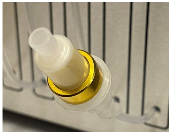
Figure 8: ATEC 8000 DNPH Cartridge Flow Check Connection Setup
