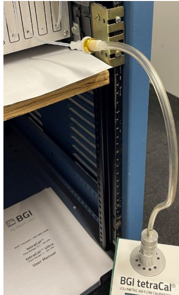
Figure 11: ATEC 8000 DNPH Cartridge Flow Check Setup
