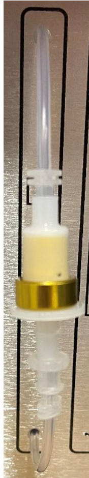
Figure 12: ATEC 8000 DNPH Cartridge Collection Setup
