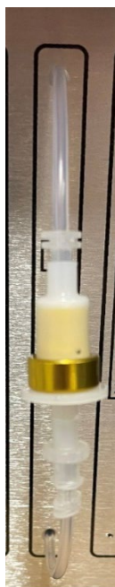
Figure 11: ATEC 8000 DNPH Cartridge Collection Setup
