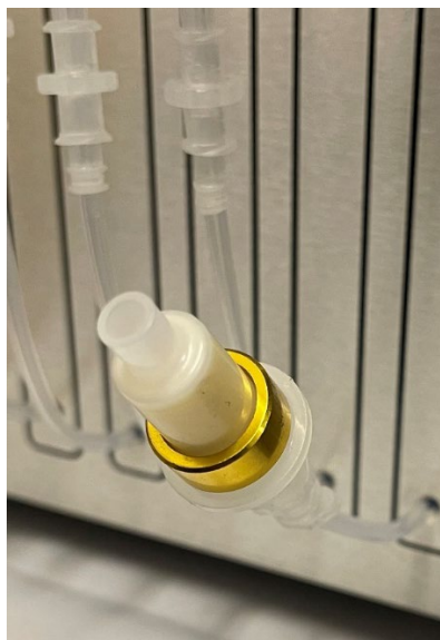
Figure 6: ATEC 8000 DNPH Cartridge Flow Check Connection Setup
