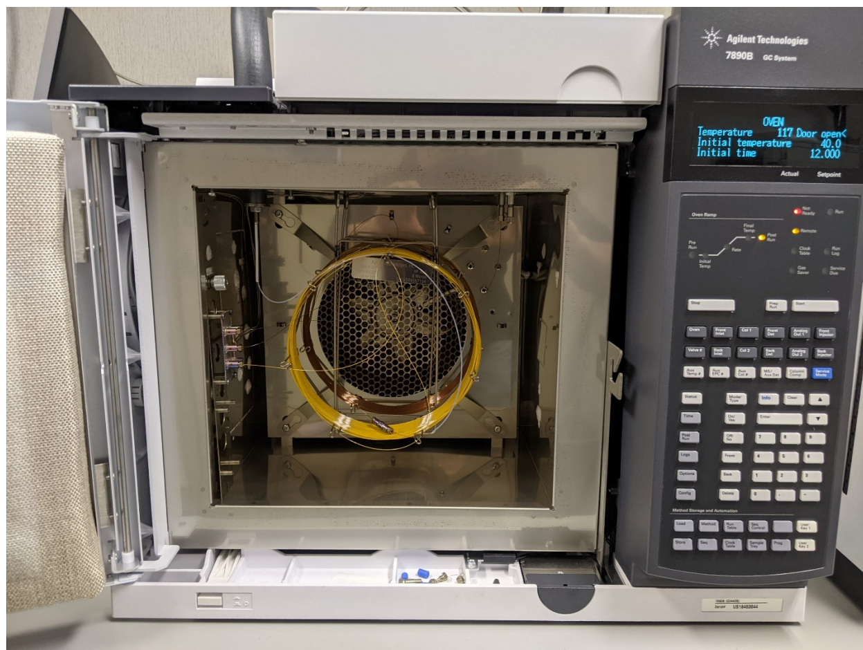
Figure 33: Agilent 7890B Oven and Column Configuration
