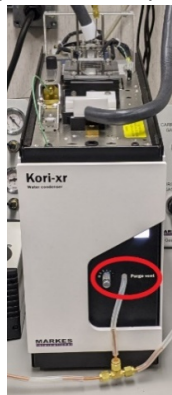
Figure 2: Kori water condenser with purge vent circled in red
