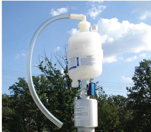
**Figure 73. HEPA Filter Assembly.**
