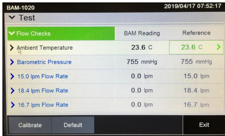
**Figure 70. Temperature and Pressure Calibration Screen.**
