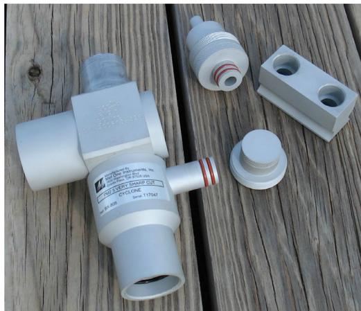
**Figure 80. Disassembled VSCC.**
