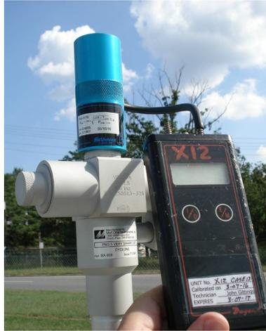
**Figure 51. FTS with Manometer.**
