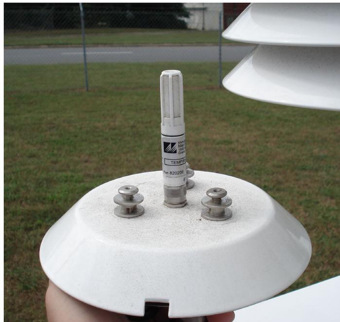
**Figure 83. Ambient Temperature Probe.**
