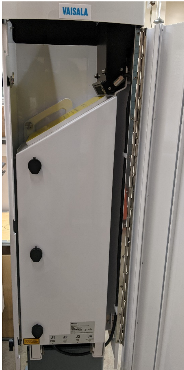
Figure 6: Vaisala CL-51 Ceilometer Instrument Window and Internals Housing
