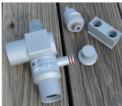
Figure 26. Disassembling the VSCC for Cleaning
