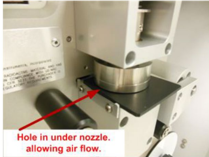
Figure 87. Leak Isolation Shim Position for Upper System Leak Test.
