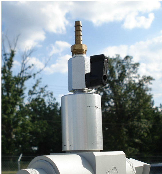
Figure 28. Flow Audit Adapter for Tetra Cal.
