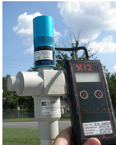
Figure 45. FTS with Manometer.
