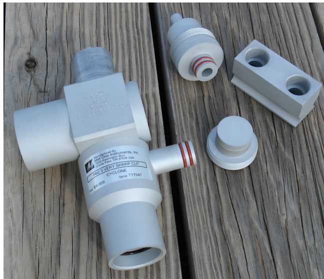
Figure 58. Disassembling the VSCC for Cleaning.
