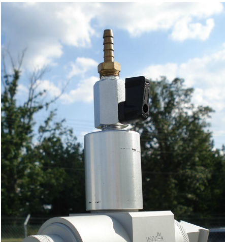
Figure 44. Flow Audit Adapter for Tetra Cal.
