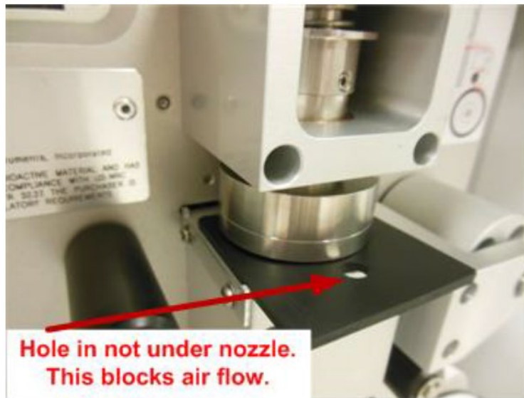
Figure 86. Leak Isolation Shim Position for Lower System Leak Test.
