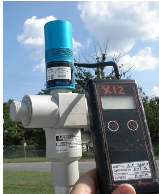
Figure 29. FTS with Manometer.
