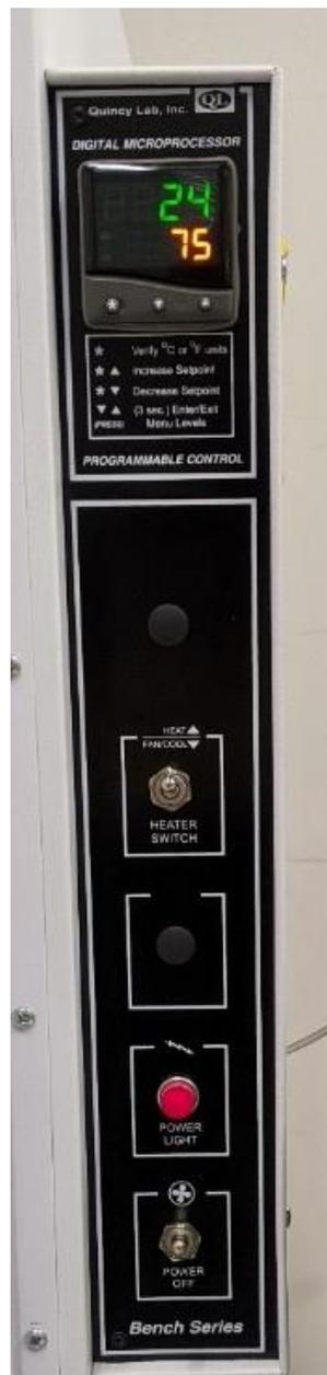
*Figure 5: Entech 3100A Canister Cleaning System Oven Control Panel*
