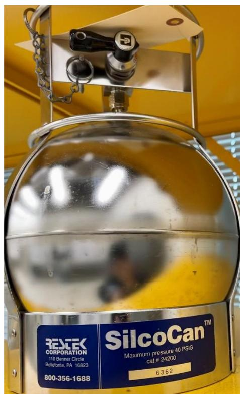
Figure 3: Restek Silco-Treated SilcoCan 6 L Canister
