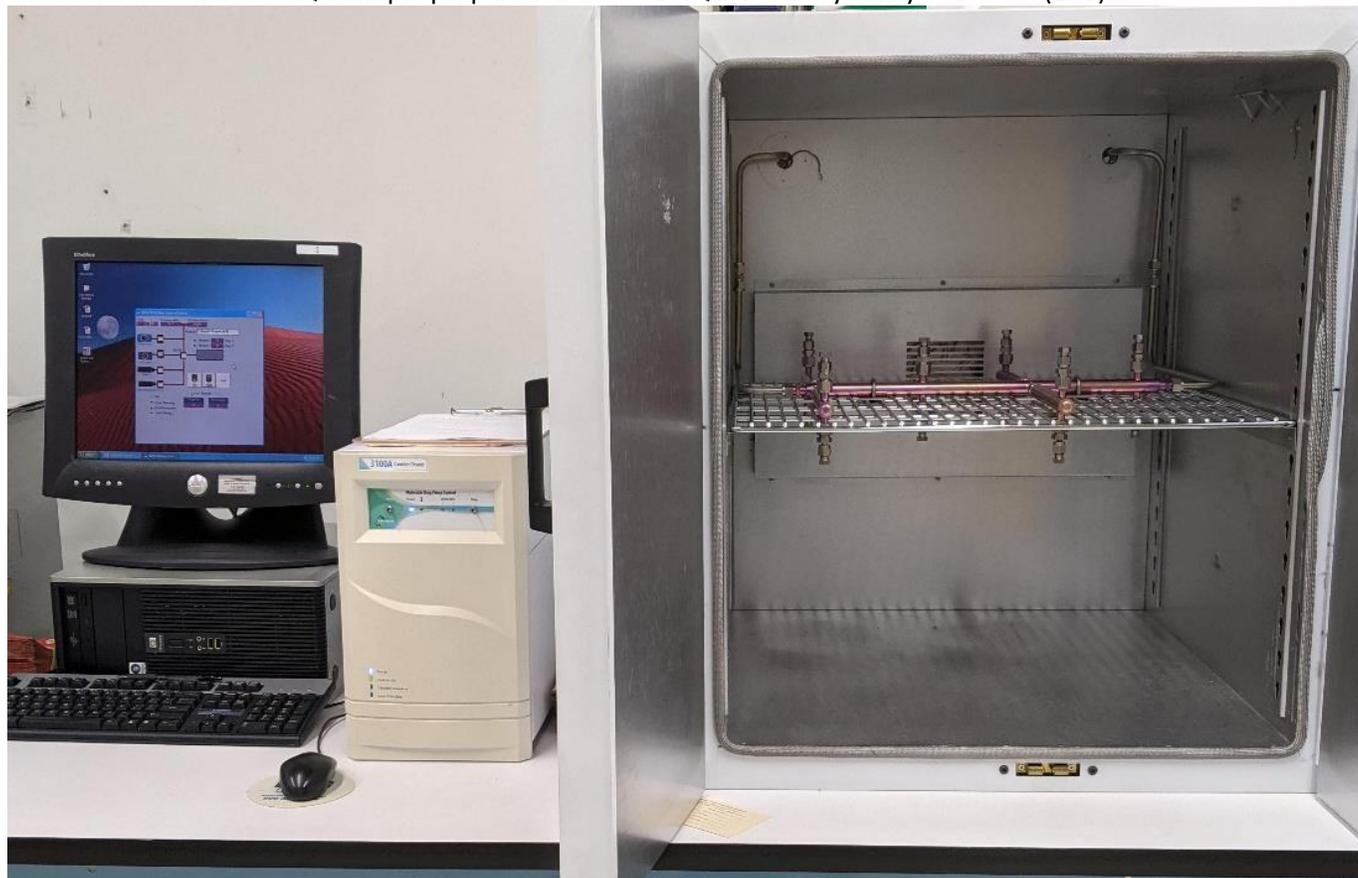
*Figure 1: Entech 3100A Canister Cleaning System*
