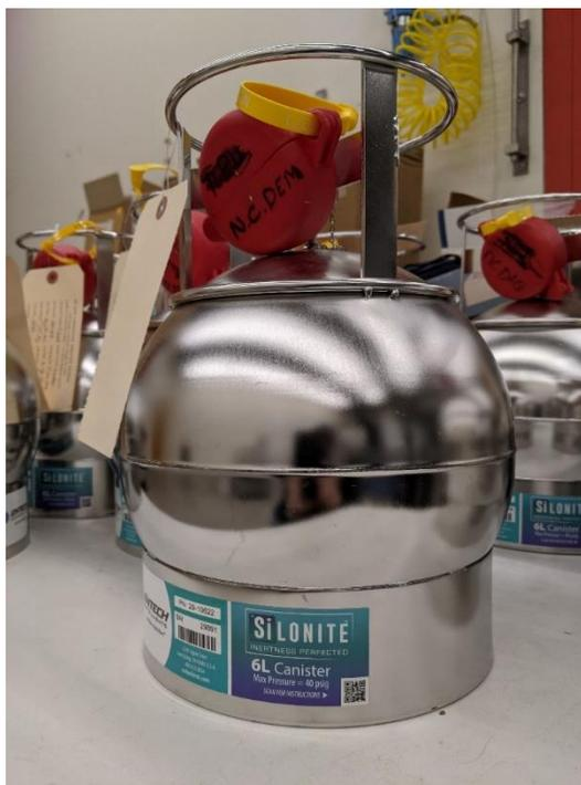
Figure 2: Entech Silonite Silco-Treated 6 L Canister
