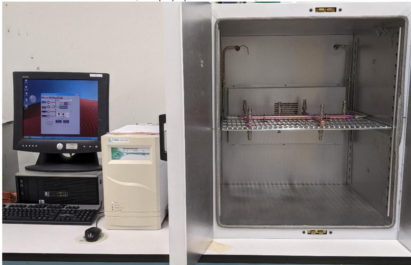
*Figure 1: Entech 3100A Canister Cleaning System*
