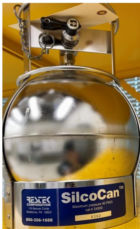
Figure 3: Restek Silco-Treated SilcoCan 6-L Canister
