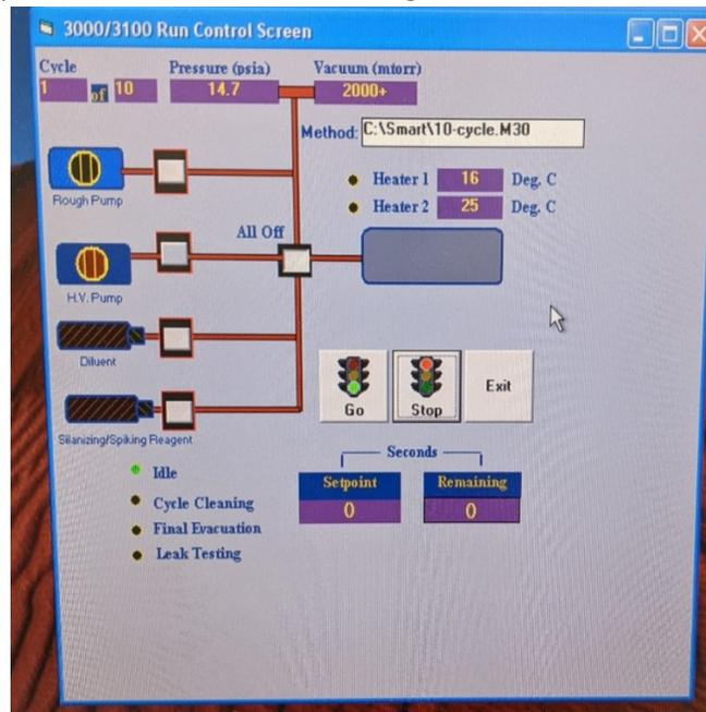
Figure 7: Entech 3100A Canister Cleaning System Run Screen
