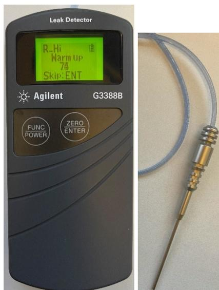
*Figure 8: Agilent G3388B Leak Detector and Probe*
