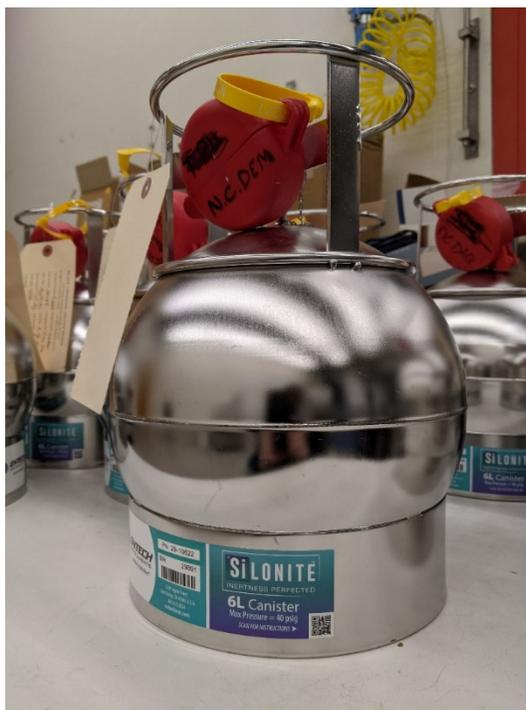
Figure 2: Entech Silonite Silco-Treated 6-L Canister
