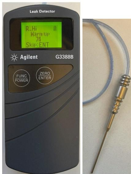
*Figure 9: Agilent G3388B Leak Detector and Probe*
