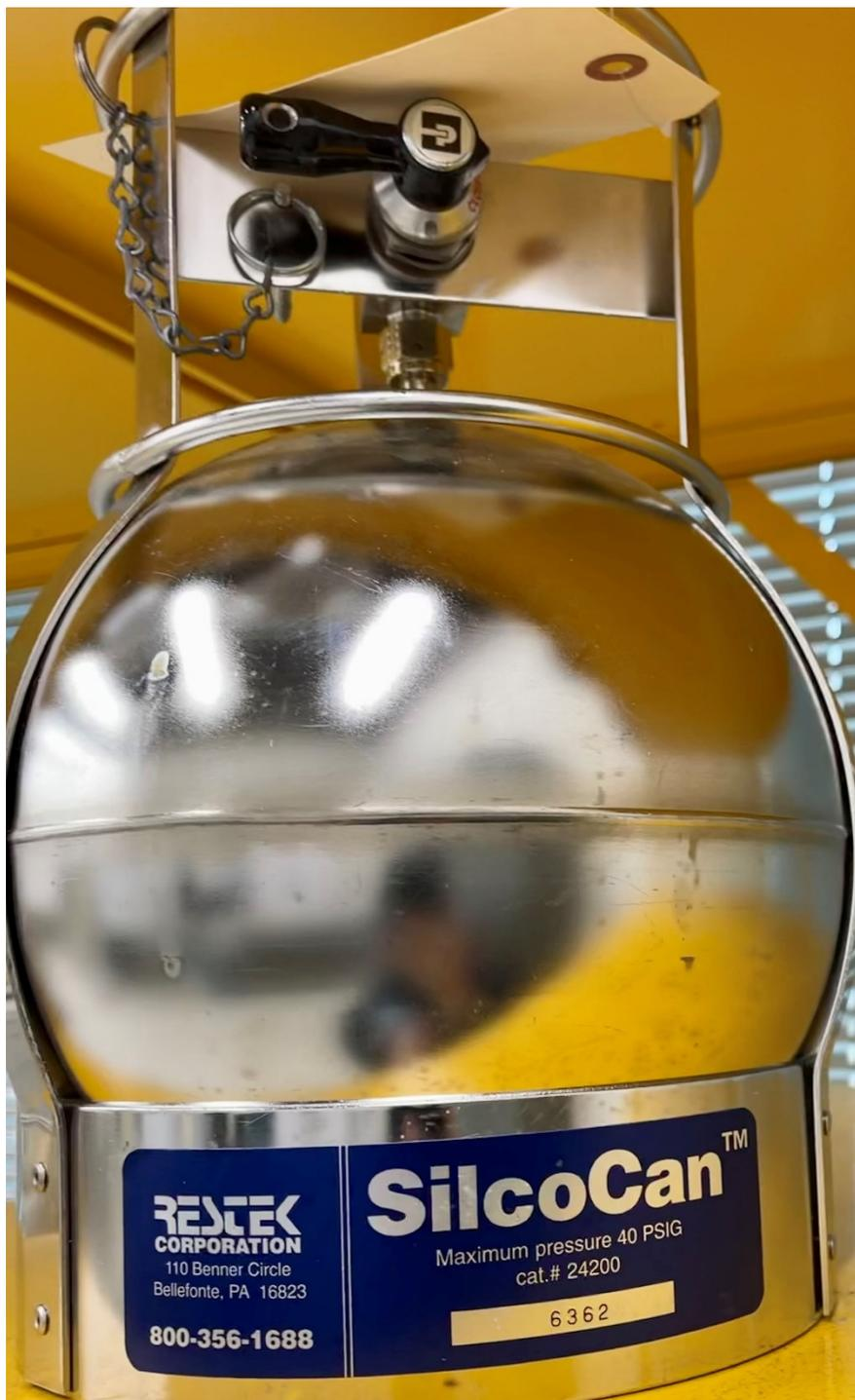
*Figure 3: Restek Silco-Treated SilcoCan 6-L Canister*
