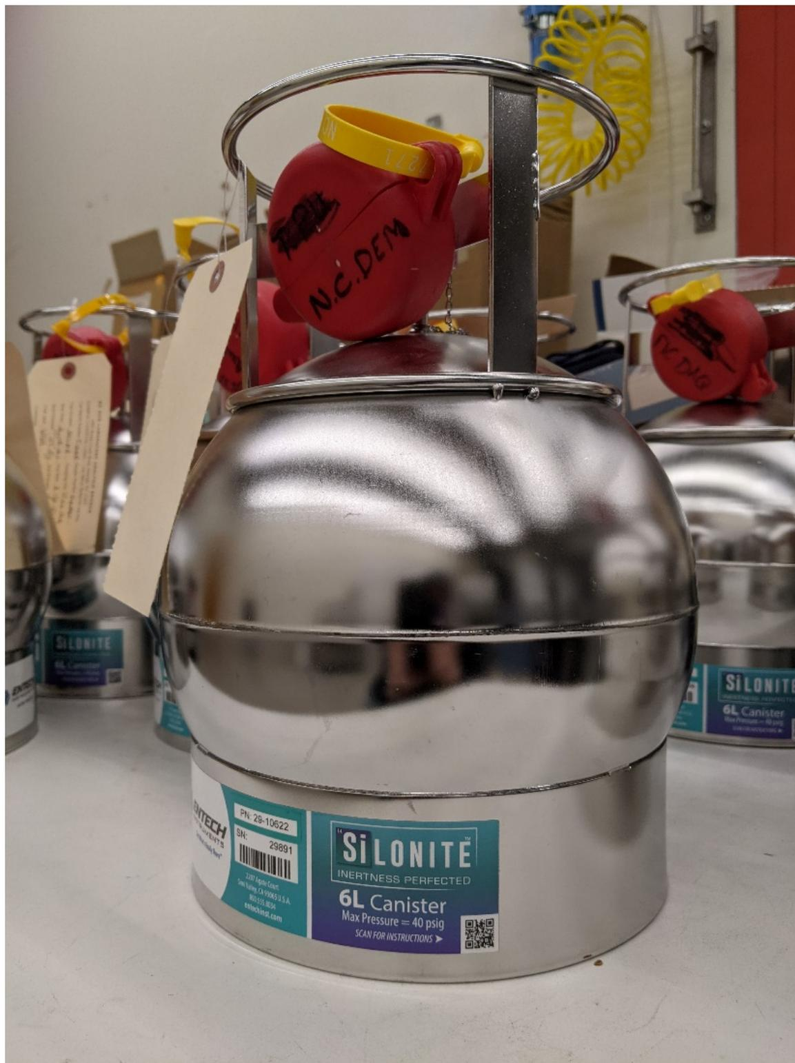
Figure 2: Entech Silonite Silco-Treated Summa 6-L Canister
