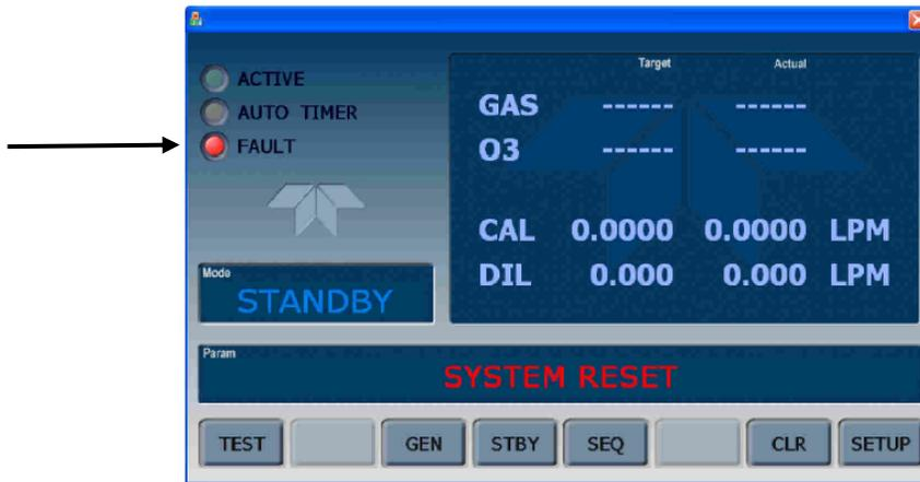
**Figure 3 T700U Calibrator Front Screen**
