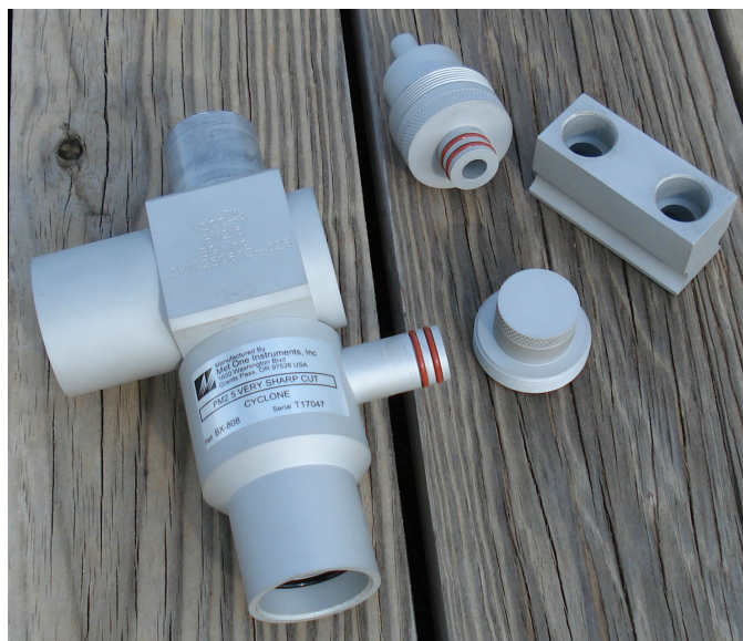
Figure 26. Disassembling the VSCC for Cleaning
