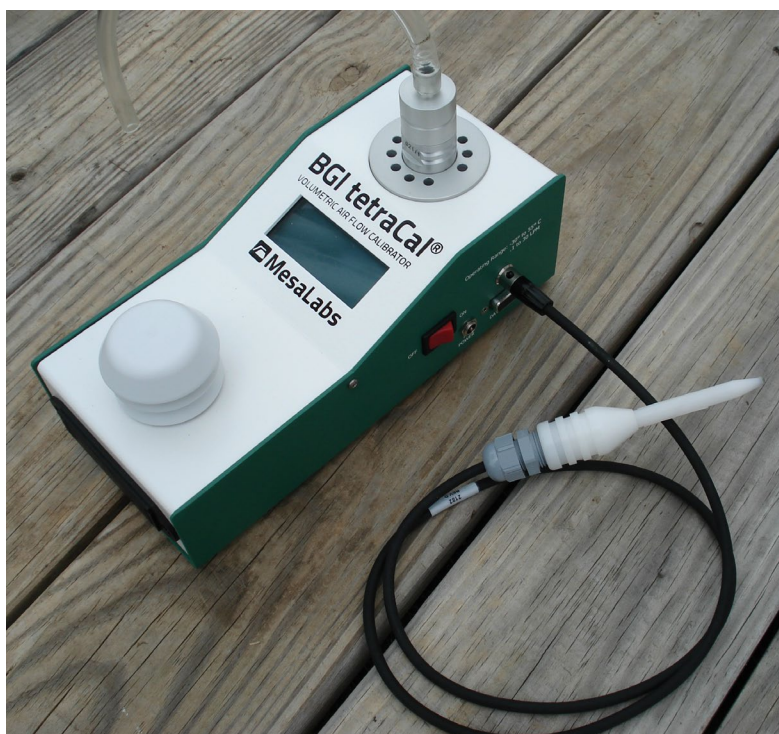
Figure 19. BGI Tetra Cal with Optional Temperature Probe.
