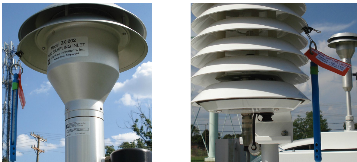
Figure 21. Proper Shaded Inlet and Solar Shield Location.
