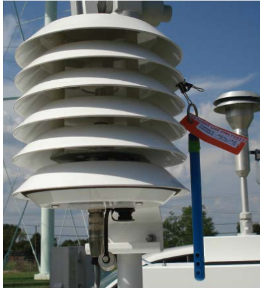
Figure 28. Proper Shaded Location.
