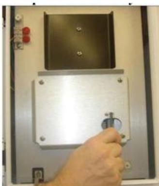
**Figure 28. Inserting the Compact Flash Memory Card**
