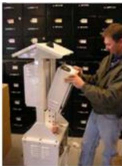
**Figure 15. Inserting the Module Boxes and the Downtube**
