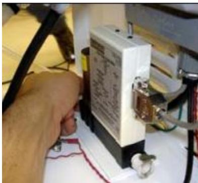
**Figure 50. Removing Rear Hose to MFC**
