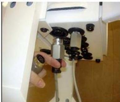
**Figure 20. Connection of the Controller Cable to Controller Module**
