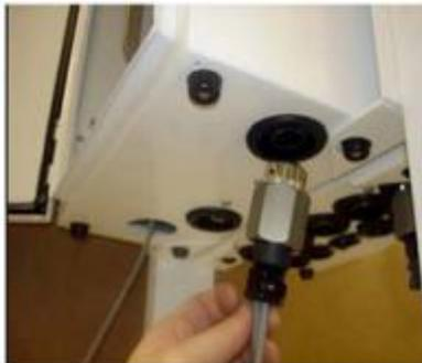
**Figure 21. Connection of the Controller Cable to Sample Module**
