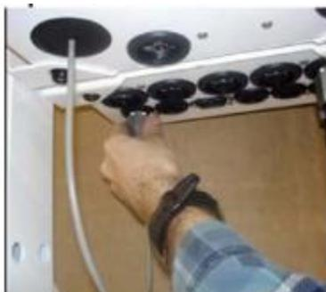
**Figure 25. Connection of the Ambient Temperature Probe to the Sample Module and Controller Module**
