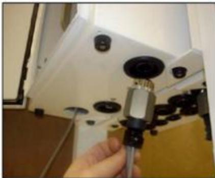
**Figure 45. Removing the Controller Cable**
