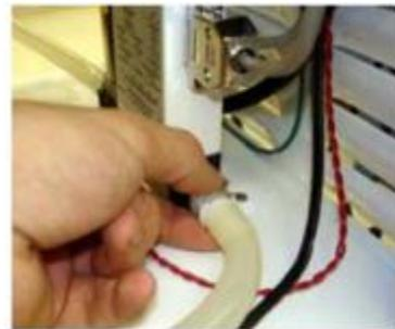
**Figure 49. Removing Front Hose on the MFC**
