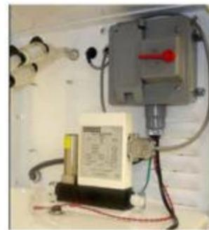
**Figure 14. Mass Flow Controller and Power Box**
