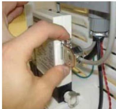
**Figure 51. Removing MFC Data Cable**
