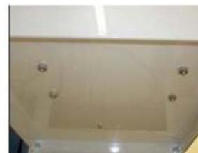
**Figure 54. Remove Nuts from Bottom of Pump Enclosure**
