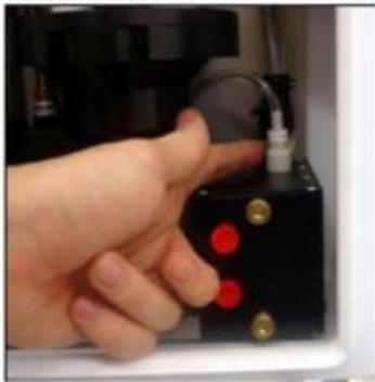
**Figure 44. Removing the Vacuum Sensor Tube**
