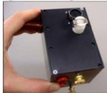
**Figure 47. Removing the Electronic Box**
