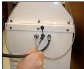
**Figure 24. Connection of Air Line to the Lower Stand (Pump Enclosure)**
