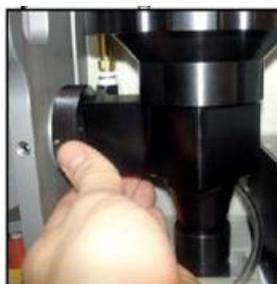
**Figure 60. Unscrewing the Cyclone Ring**
