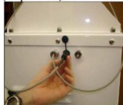
**Figure 22. Connection of the Controller Cable to Mass Flow Controller Connection on Lower Stand (Pump Enclosure)**
