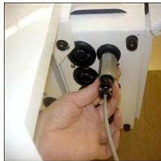
**Figure 19. Connection of the Pump Relay Cable to bottom of Controller Module**
