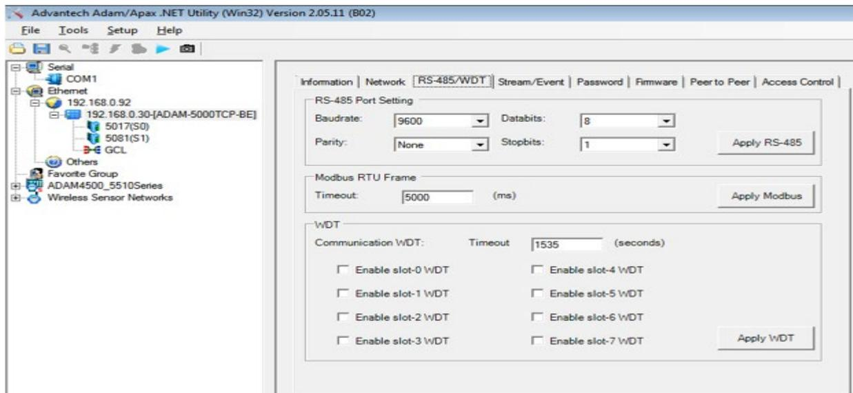
Figure 5 - Solar Radiation Sensor RS-485/WDT Port Settings.
