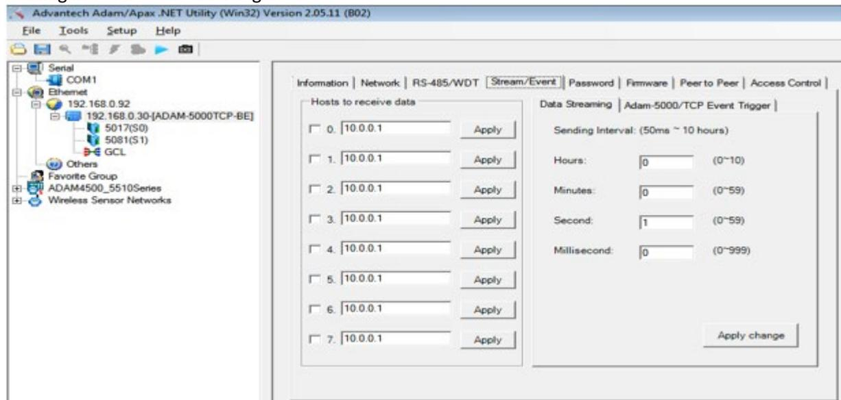
Figure 6 - Solar Radiation Sensor Stream/Event Configuration
