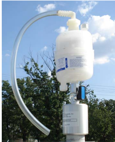
Figure 29. Leak Check Adapter with HEPA Filter.
