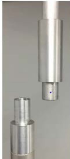
Figure 18. Slip Coupler Moved to the Side to Allow Monitor Use with Audit Devices.
