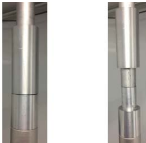
Figure 17. Slip Coupler in Normal Position and Lifted Vertically.
