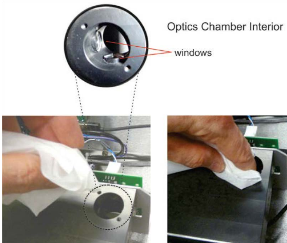
Figure 47. Optics Chamber Windows.
