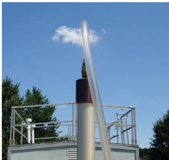
Figure 32. Flow Audit Adapter with Flow Standard Connected.
