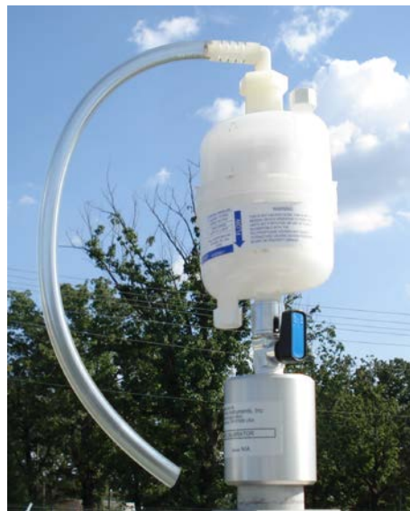
Figure 16. Leak Check Adapter with HEPA Filter.
