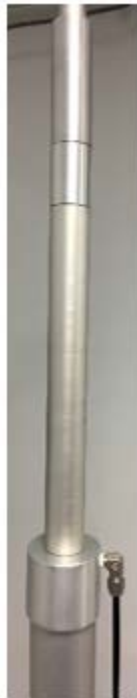
Figure 41. Extension Tube and Upper Inlet Tube Over the ASC.
