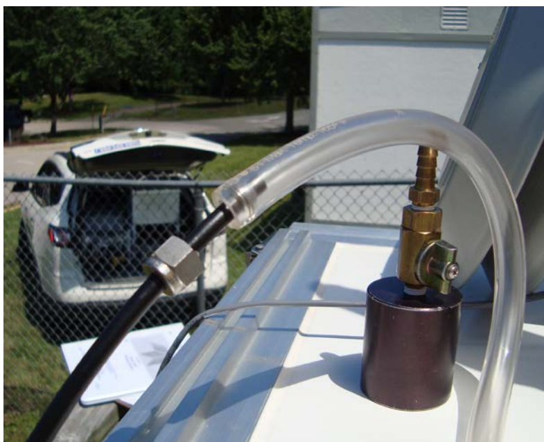
Figure 23. Flow Standard Connected to the Bypass Line.
