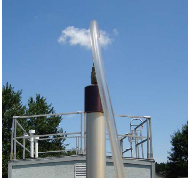
Figure 25. Flow Audit Adapter with Flow Standard Connected.
