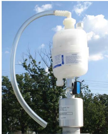
Figure 26. Leak Check Adapter with HEPA Filter.
