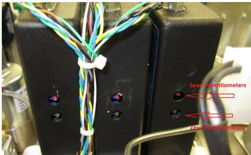
**Figure 4.4 Zero and Span Potentiometers for Mass Flow Meters**
