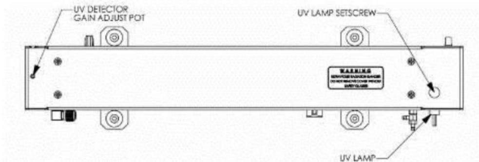
**Figure 8.2 Photometer Assembly – Lamp Adjustment / Installation**
