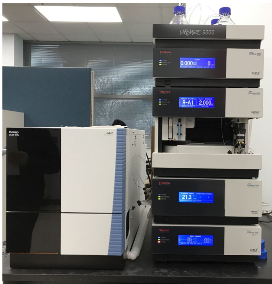
Figure 1: Thermo Ultra High-Performance Liquid Chromatograph with Ultra-Violet Radiation Detector and Mass Spectrometer
