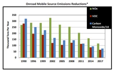
\* The NOx emissions spike in 2002 is attributed to EPA adjusting the anroad emissions model.
