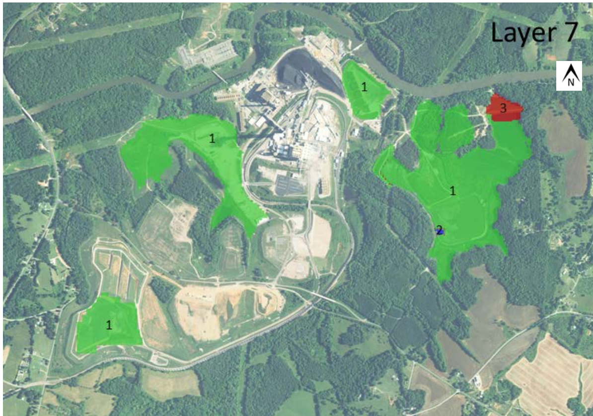
Figure 5-1g. Zones used to define horizontal hydraulic conductivity and horizontal to vertical anisotropy in the ash (model layer 7 shown). Blue regions are areas with high conductivity to represent future closure scenarios where ash would be stacked. The remainder of ash basins have conductivities of 2 ft/d.
