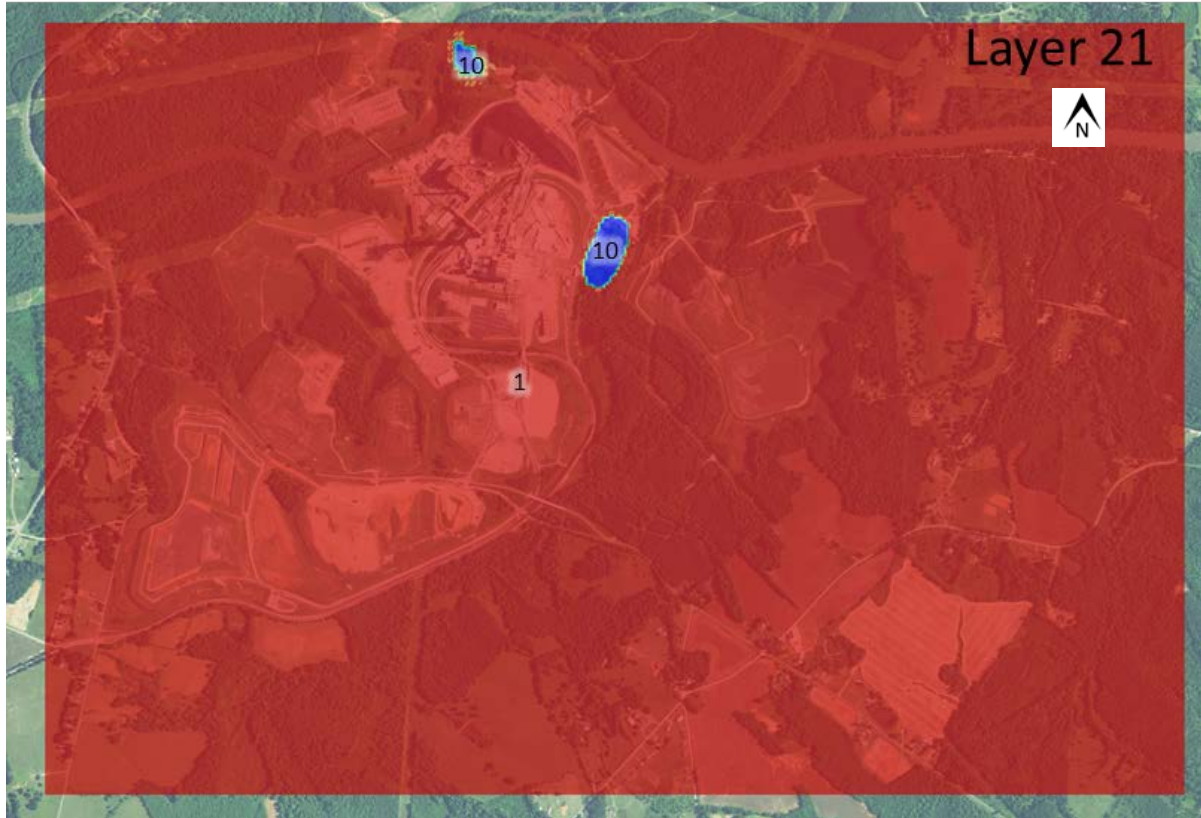
Figure 5-6a. Zones used to define horizontal hydraulic conductivity and horizontal to vertical anisotropy in the bedrock, model layer 21.
