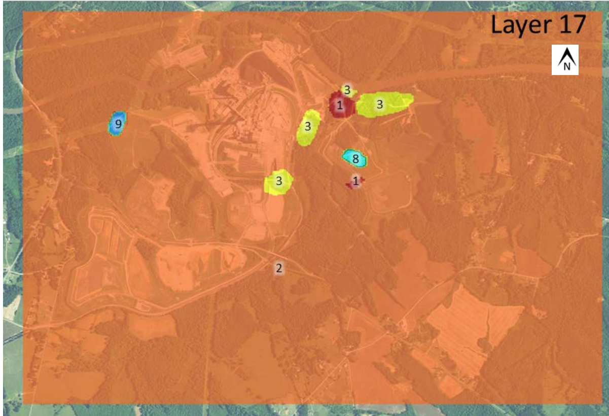
Figure 5-5a. Zones used to define horizontal hydraulic conductivity and horizontal to vertical anisotropy in the upper bedrock, model layer 17.
