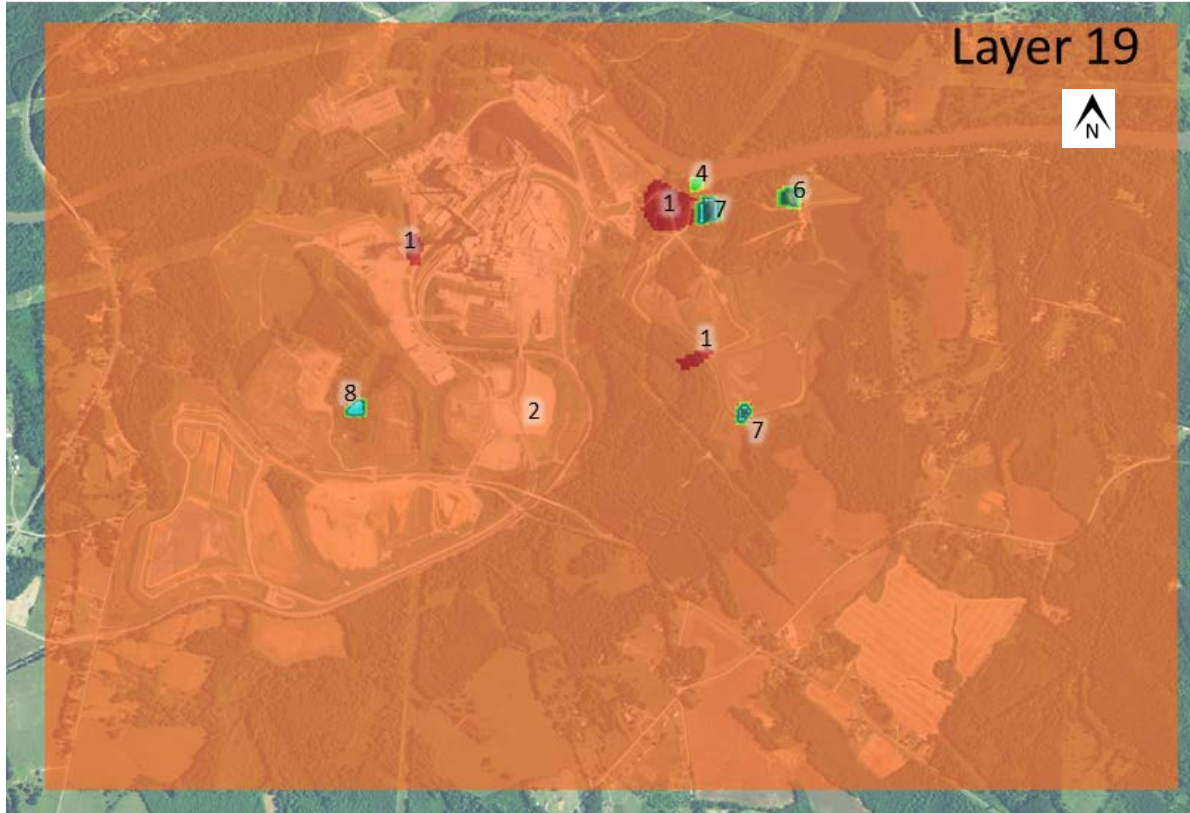
Figure 5-5c. Zones used to define horizontal hydraulic conductivity and horizontal to vertical anisotropy in the upper bedrock, model layer 19.
