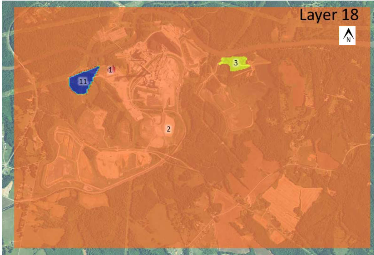
Figure 5-5b. Zones used to define horizontal hydraulic conductivity and horizontal to vertical anisotropy in the upper bedrock, model layer 18.
