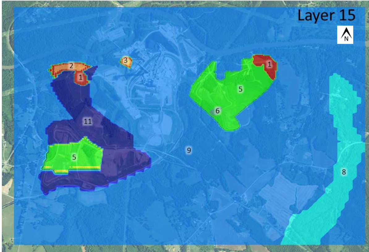
Figure 5-3b. Zones used to define horizontal hydraulic conductivity and horizontal to vertical anisotropy in the transition zone, model layer 15.
