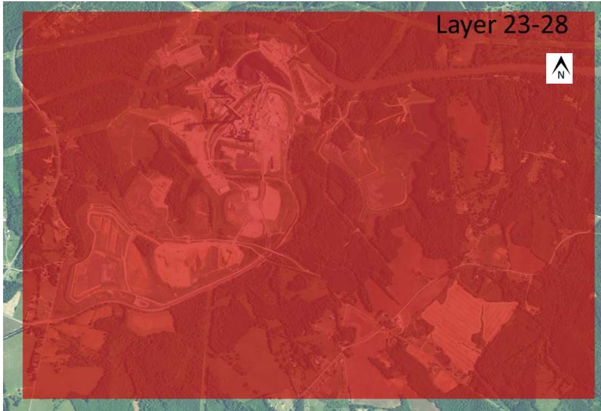
Figure 5-7. Zones used to define horizontal hydraulic conductivity and horizontal to vertical anisotropy in the deep bedrock, model layers 23-28.
