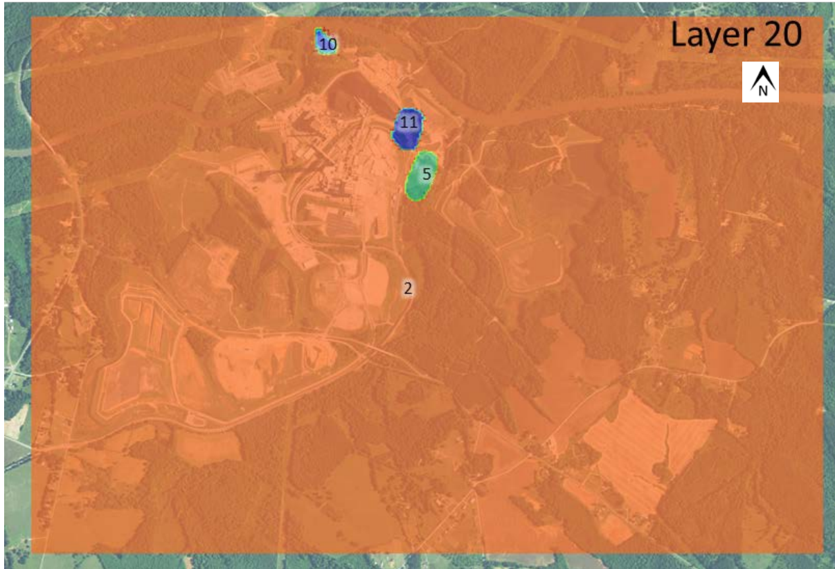
Figure 5-5d. Zones used to define horizontal hydraulic conductivity and horizontal to vertical anisotropy in the upper bedrock, model layer 20.
