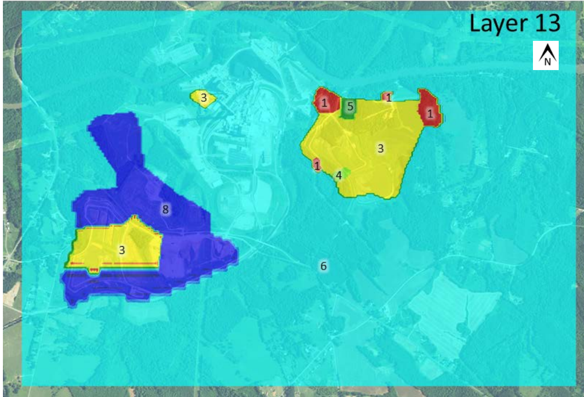
Figure 5-2d. Zones used to define horizontal hydraulic conductivity and horizontal to vertical anisotropy in the upper saprolite, model layer 13.
