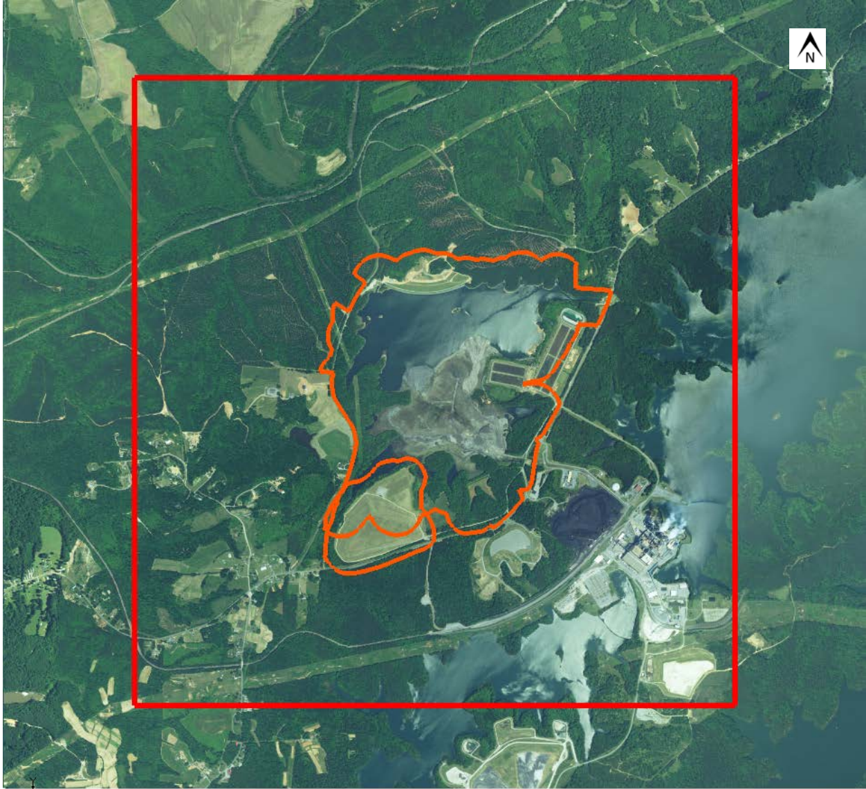
Figure 4-1. Numerical model domain. Domain is represented as the red square. The larger orange outline is the ash basin compliance boundary and the smaller orange outline is Pine Hall Road Landfill.
