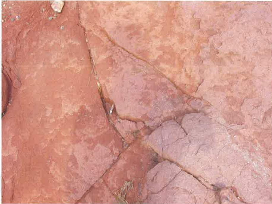
Photograph 3. View of muddy sandstone at the layered rock exposure. Note the near vertical fractures oriented \sim N 10^\circ E and \sim N 60^\circ W.
