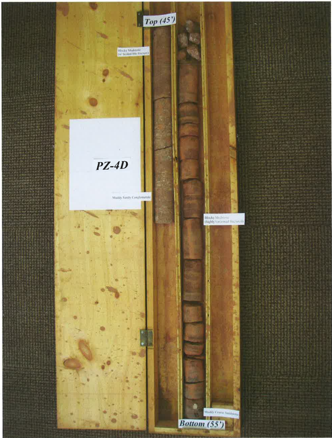
View of rock core PZ-4D from 45 feet to 55 feet below grade. 1 st Run (left) and 2 nd Run (right).
