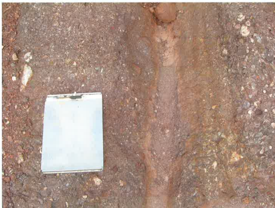
Photograph 2. View of the muddy conglomerate located at the rock outcrop. Note the linear excavation equipment claw mark.
