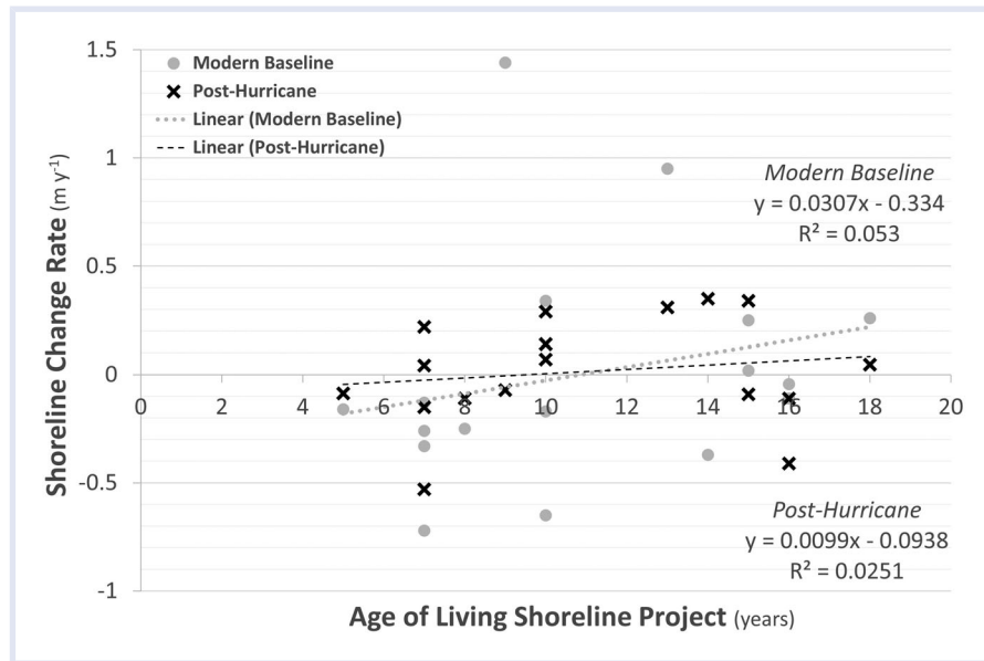
FIGURE 4 The effect of age of living shoreline projects (x-axis) in years on shoreline change rate (SCR; y-axis) in meters per year. The scatterplot shows the long-term SCR of shorelines of various ages from their installation to before Hurricane Florence (gray circles). It also shows the change in short-term SCR after Hurricane Florence (black cross). There is a slight positive correlation between age and SCR, this correlation decreased after Hurricane Florence, showing that with age there may be increasing resilience among living shoreline projects
