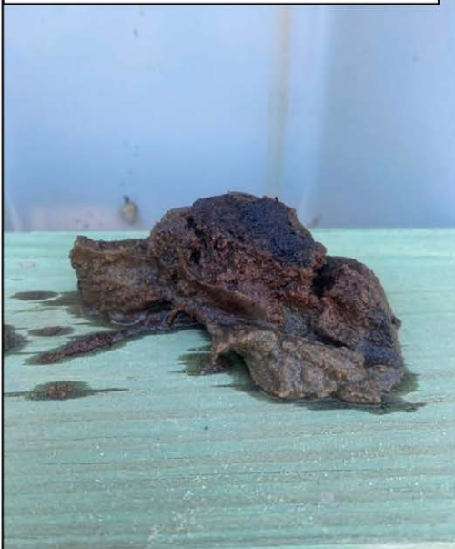
Photo #3 (3/7/23) – Core sample illustrating substrate within the area of the proposed floating platform.
