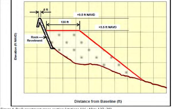
Figure 4. Rock revetment cross-section (stations 116+40 to 137+20)
