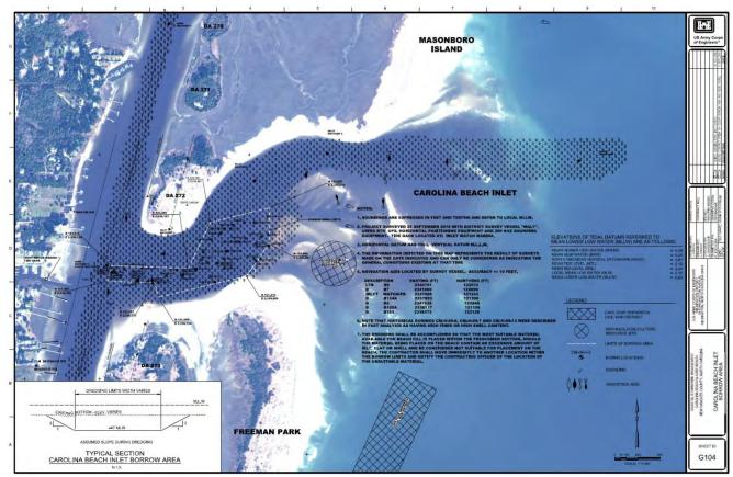
Figure 7. Carolina Beach Inlet Sediment Trap/Borrow Area
