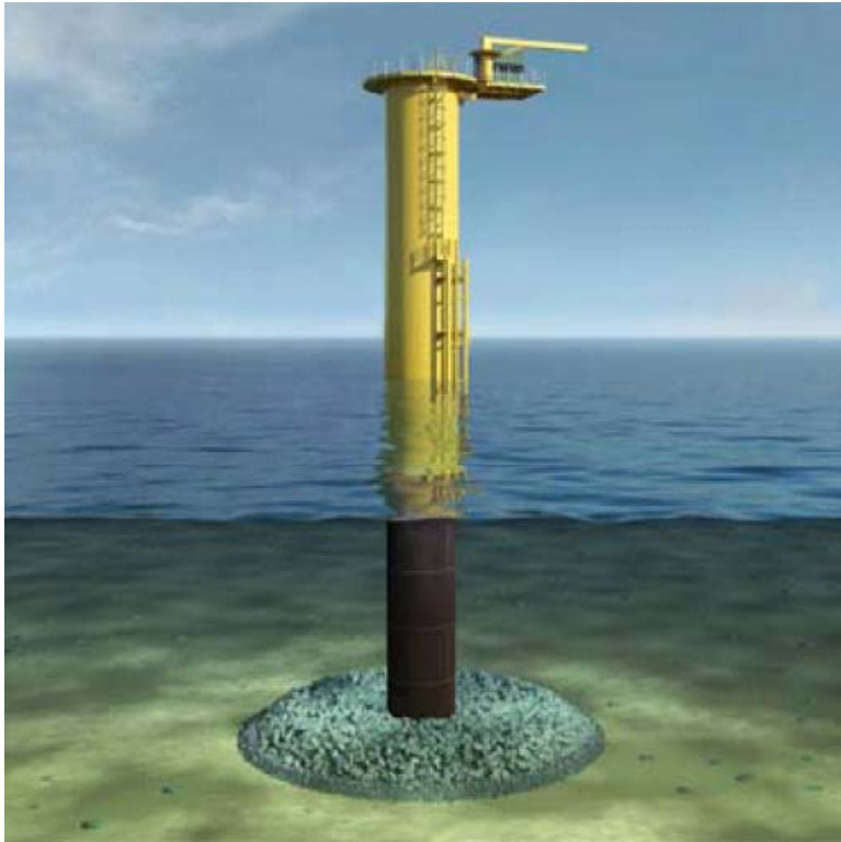
Monopile foundation with transition piece and scour protection. Flange height above sea level approximately 20 meters.
