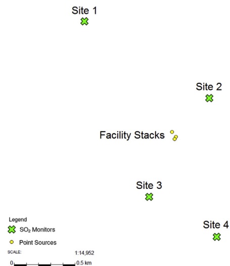
Fig. 3. At left, the industrial facility point source emissions in relation to \text{SO}_2 ambient air monitor locations.
