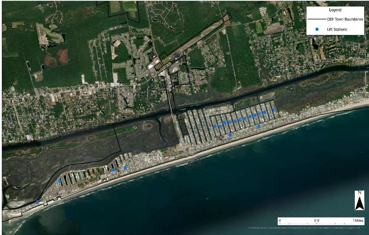
Figure 2. Lift stations identified for control panel elevation. Transformer pedestals are approximately co-located with the lift stations.
