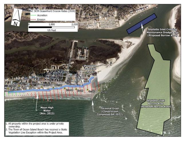
Figure 1. Project location map showing the location of the Shallotte Inlet Crossing and Shallotte Inlet borrow areas, Mean High Water Line, and the NC DCM Erosion Rates (Figure courtesy of Town of Ocean Isle Beach).
