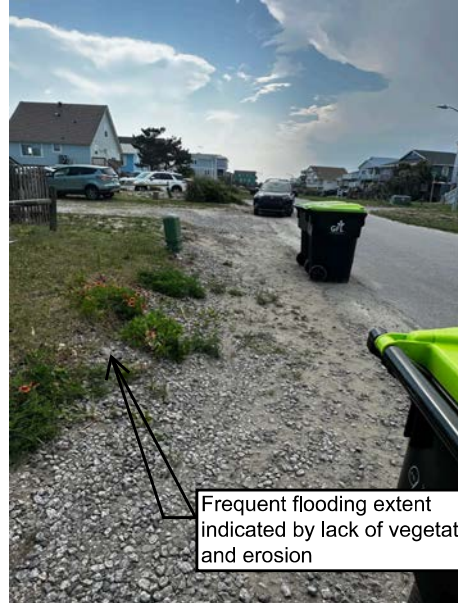
Photo 21: Flooding extends into driveways on land side of Ocean Dr
