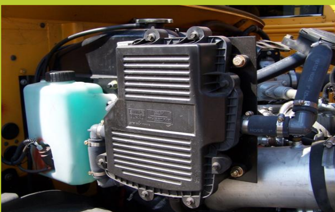
The two methods of emission reduction for the CCS busses came in the forms of Diesel Oxidation Catalysts (above) and Closed Crankcase Ventilation Systems (below).
