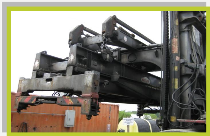
The four point top pick loaded container attachment with twistlock interlocks on the four corners is used to move loaded containers from one location to another.
