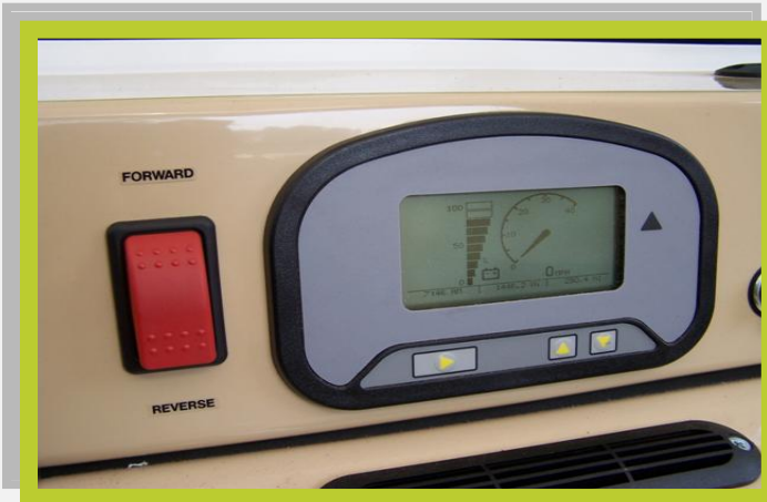
The Patriot comes equipped with a speedometer, battery discharge indicator, hour meter and other digital features (above) and is capable of easy navigation around the HCC campus (below).
