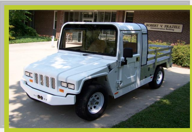
This model of the EXV2 Patriot has heavy duty aluminum stake sides, allowing it to transport more of the college's trash and recycling per pickup.
