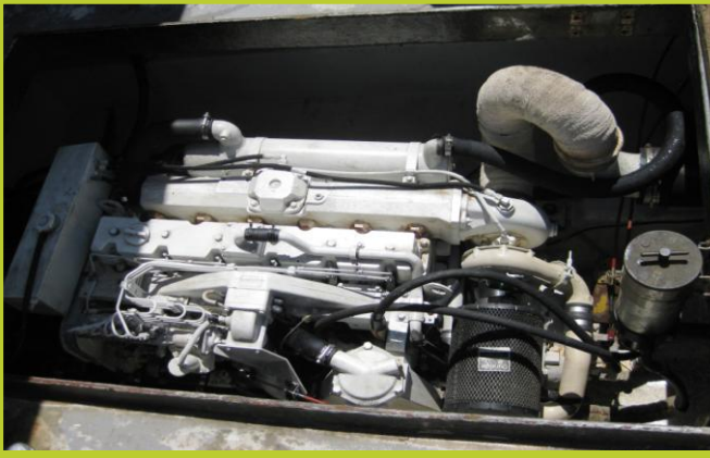
The new 2012 Cummins 6CTA8.3M2, 430 horsepower, V6 diesel engine. With its Tier 2 rating, hazardous diesel emissions have greatly decreased for Mr. Sadler.
