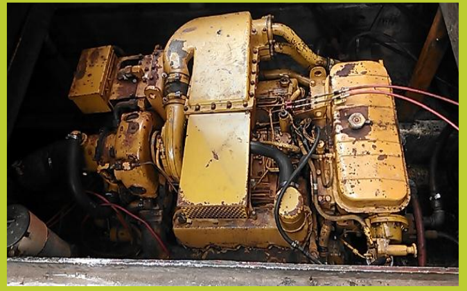
The old unregulated 1990 Caterpillar 3208 with a 435 horsepower, 4 cycle, V8 diesel engine was replaced with the new engine (to the left).
