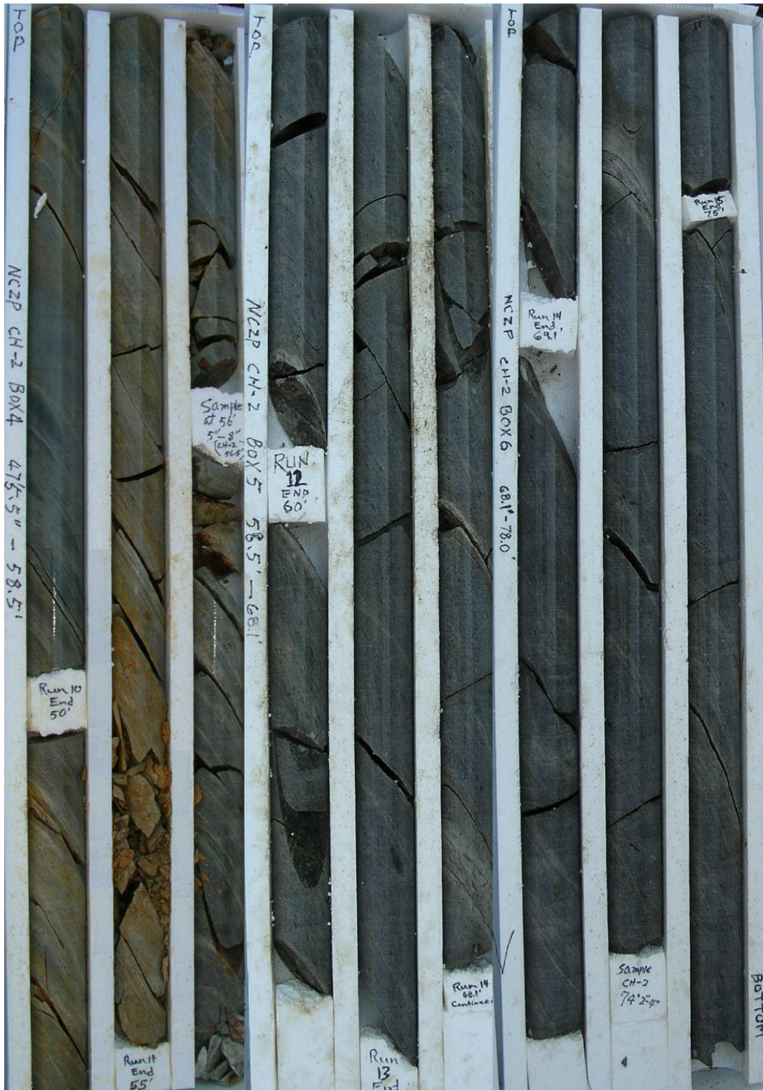
Figure 5. Example of core: Core sample from CH-2 at the NCZGMRS showing fracture characteristics and weathering conditions of the bedrock
