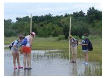
Students measuring the horizontal distance with metric tape measure.
