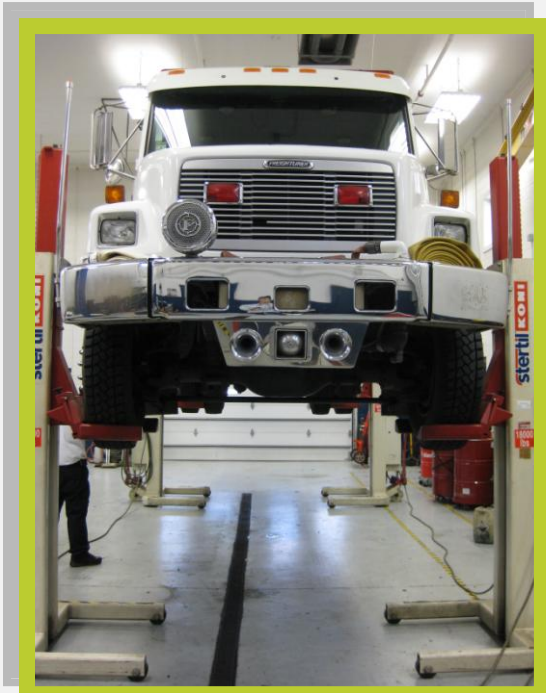
Skyland Fire Department's 1996 Freightliner FL80 Diesel Fire Engine (left). It was lifted about six feet in the air to better view the Diesel Oxidation Catalyst (DOC) retrofit.
