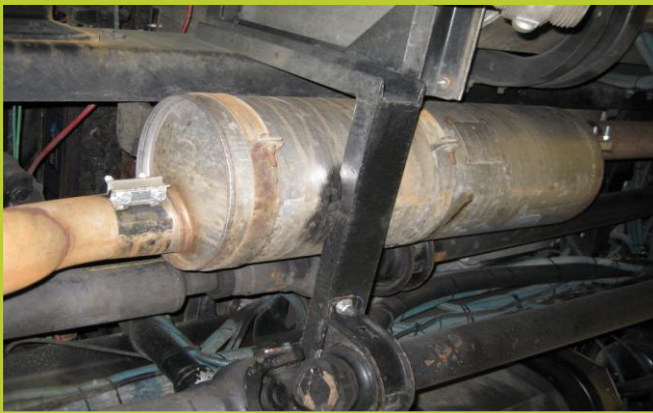
The DOC (above) can either replace the muffler or be added to the existing exhaust system.
