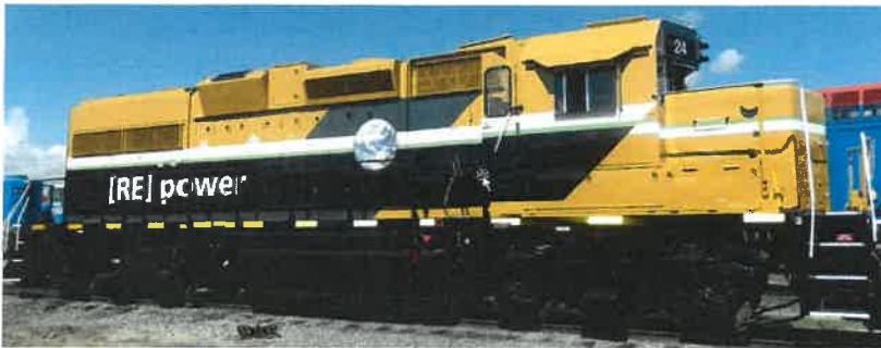
Remanufacture Switch Locomotive EMD24 to Tier 4
