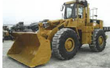
966 Loader, Unregulated to Tier 4 Total cost effectivity: $ 4,204/Ton NOx Partial cost effectivity: $ 1,682/Ton NOx
