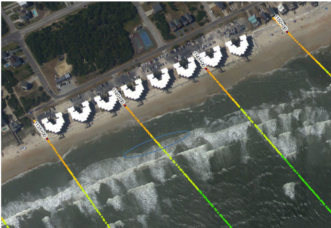
Figure 8: Post-Isaias aerial showing transect monitoring stations at the Topsail Reef Complex. Stations 1140+00 and 1145+00 front the complex.
