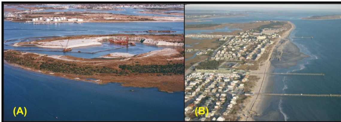
Figure 5. Historical photographs of the Brandt Island Pump-Out process. (Panel (A) - Excavation of Brandt Island utilizing a cutter-head suction dredge in 1994. Panel (B) – Active disposal of Brandt Island material to the beaches of Atlantic Beach in 2004. The former Triple S, Oceanna, and former Sportsmans Piers are located in succession from the top (east) towards the bottom (west) of the photograph.)
