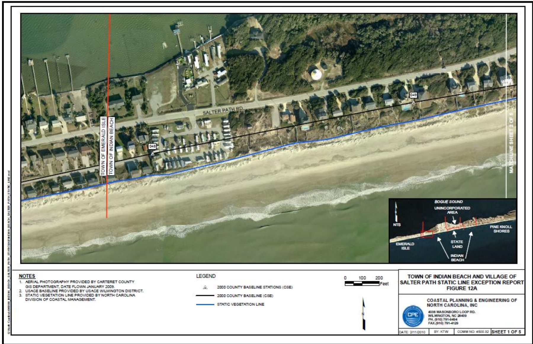
Figure 12a Indian Beach/Salter Path Static Line & Project Baseline.
