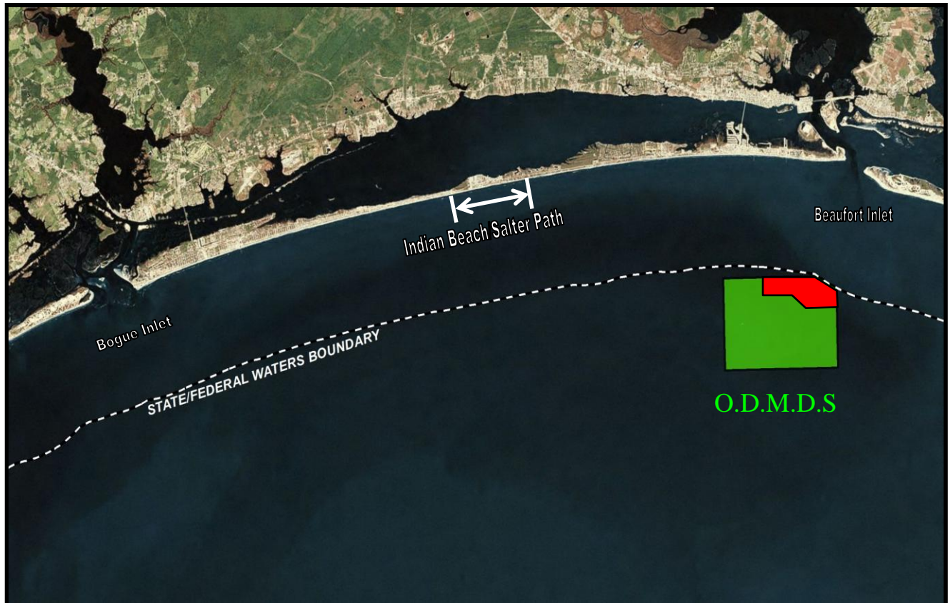
Figure 14. Morehead City Harbor Offshore Dredged Material Disposal Site (ODMDS) with area used for post-storm restorations shown in red.
