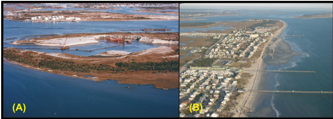
Figure 5. Historical photographs of the Brandt Island Pump-Out process. (Panel (A) - Excavation of Brandt Island utilizing a cutter-head suction dredge in 1994. Panel (B) – Active disposal of Brandt Island material to the beaches of Atlantic Beach in 2004. The former Triple S, Oceanna, and former Sportsmans Piers are located in succession from the top (east) towards the bottom (west) of the photograph.)
