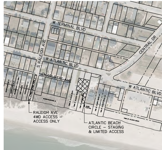
STAGING & ACCESS SITE 8 NOT TO SCALE
